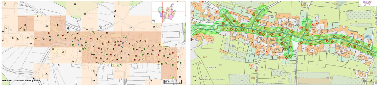
Figure 3. Thermal density mapping (left) and district heating network with buildings (right) of Meride
